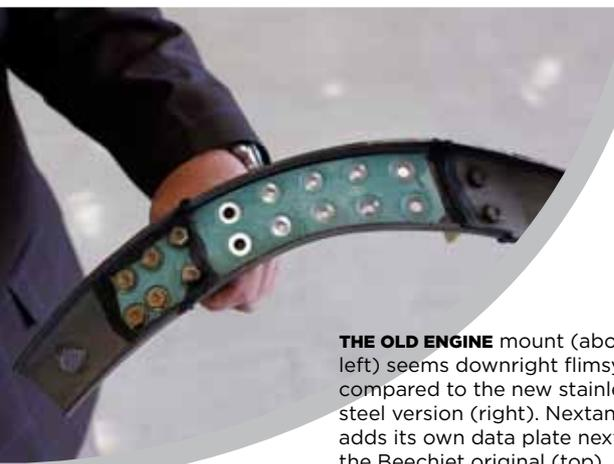
**THE OLD ENGINE** mount (above left) seems downright flimsy compared to the new stainless steel version (right). Nextant adds its own data plate next to the Beechjet original (top).
