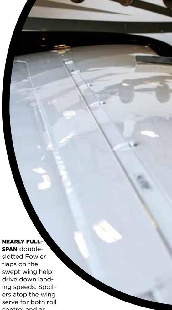
**NEARLY FULL-SPAN** double-slotted Fowler flaps on the swept wing help drive down landing speeds. Spoilers atop the wing serve for both roll control and as speed brakes.
